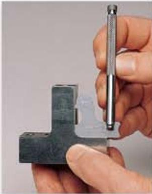
Left: Checking a radius with a 167-3/16" Radius Gage attached to a 110 Holder
