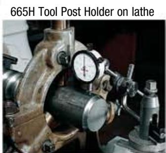
665H Tool Post Holder on lathe
