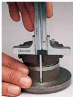
Depth Measurement with Optional Depth Attachment
